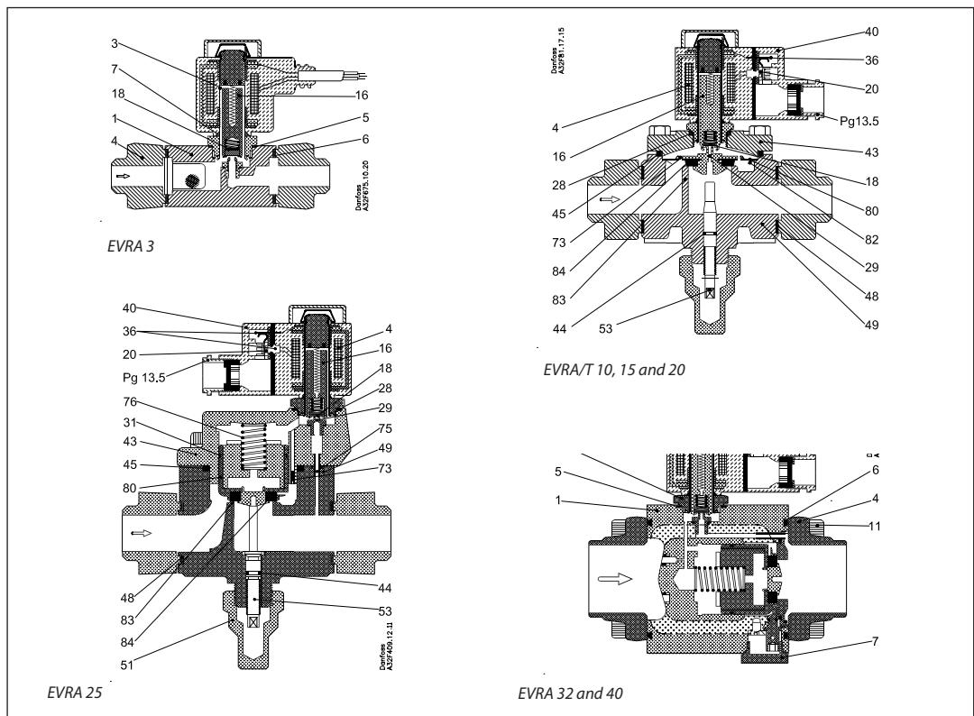
EVRA solenoid valves are designed on two different principles:
